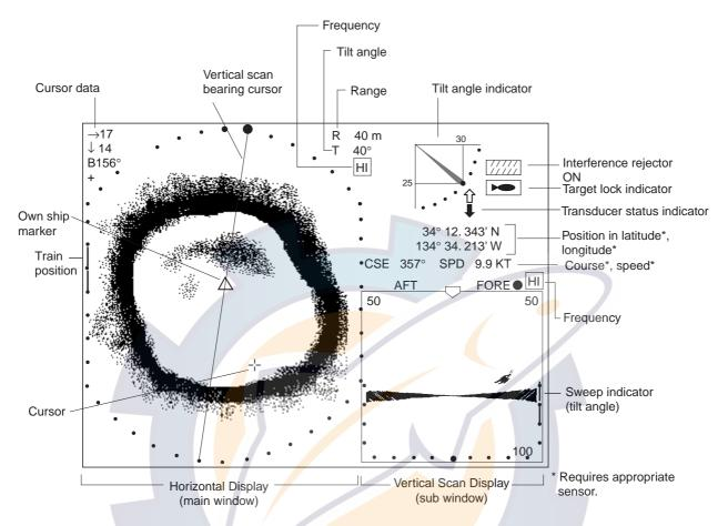
Horizontal/vertical scan display (port-starboard direction)
