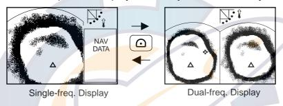
Switching between single-frequency horizontal expansion and dual-frequency horizontal expansion displays
