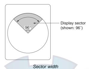
The **SECTOR** control chooses the width of the scanned sector among the sixteen positions shown in the table below. Clockwise rotation of the control increases the sector width; counterclockwise rotation decreases it.
