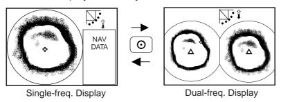
Switching between single-frequency horizontal and dual-frequency horizontal displays
