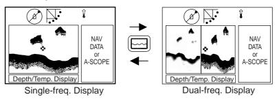
Switching between single-frequency echo sounder and dual-frequency echo sounder displays
