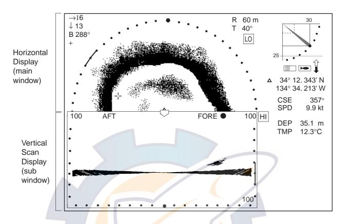
Horizontal/vertical scan display (upward-downward direction)
