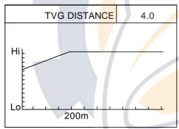
4. Press ◀ or ▶ to adjust TVG distance between 3.0 and 5.0 (130-320 m). As a general rule, use a higher setting for low-frequency transducer; a lower setting for high frequency transducer. The larger the figure the greater the distance at which TVG works. When you open the TVG dialog box the TVG line changes from solid to dashed and a solid line denotes current TVG setting.
